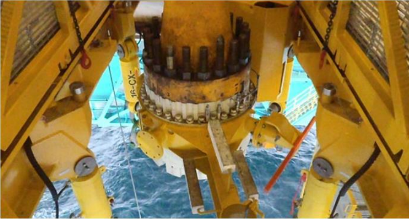
HP riser ready for launch offshore.
